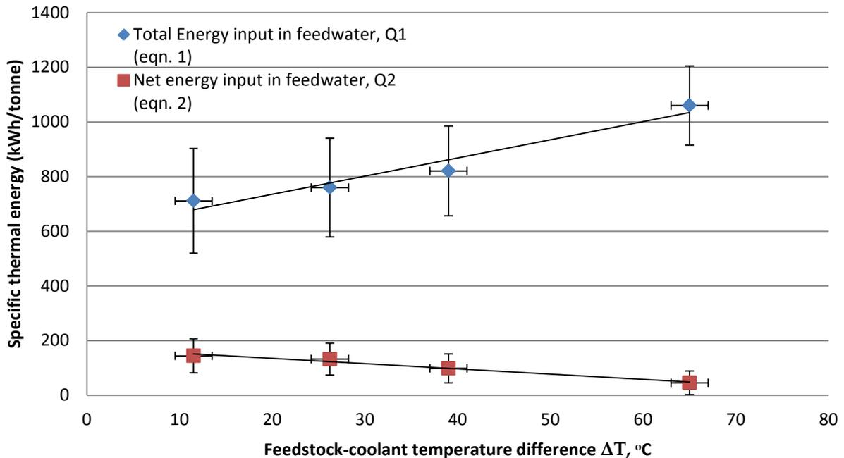
**Figure 3-3: Specific thermal energy consumption for AGMD module (feed water flow 3.8 L/min, coolant flow 1.9 L/min, feedwater temperature ca 80 °C, coolant temperature varying)**
