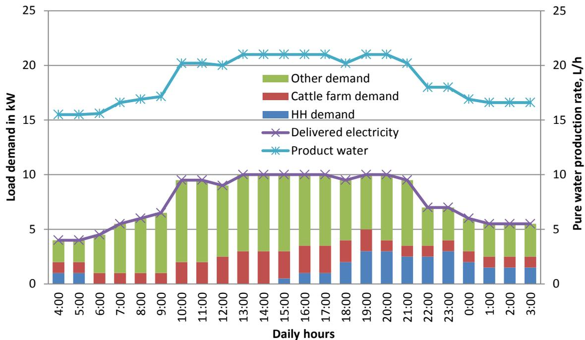
**Figure 5-1: Hourly average electricity demand proposed community and electricity supplied by biogas and pure water production of integrated system**
