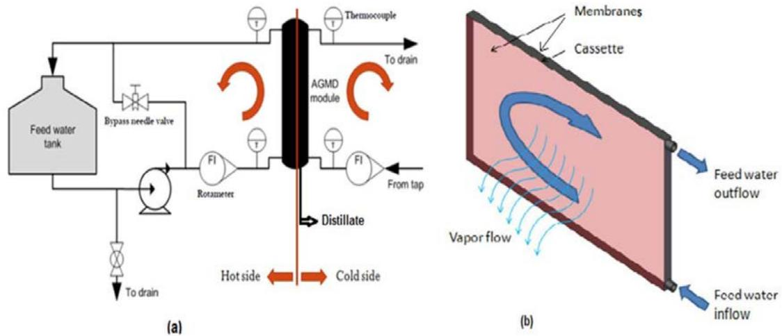
**Figure 3-1: (a) MD bench scale unit setup at KTH, (b) Membrane cassette (MD)**
