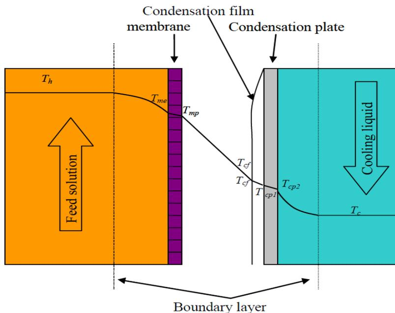
**Figure 4-2: Cross-section AGMD [Kullab and Martin, 2011]**
