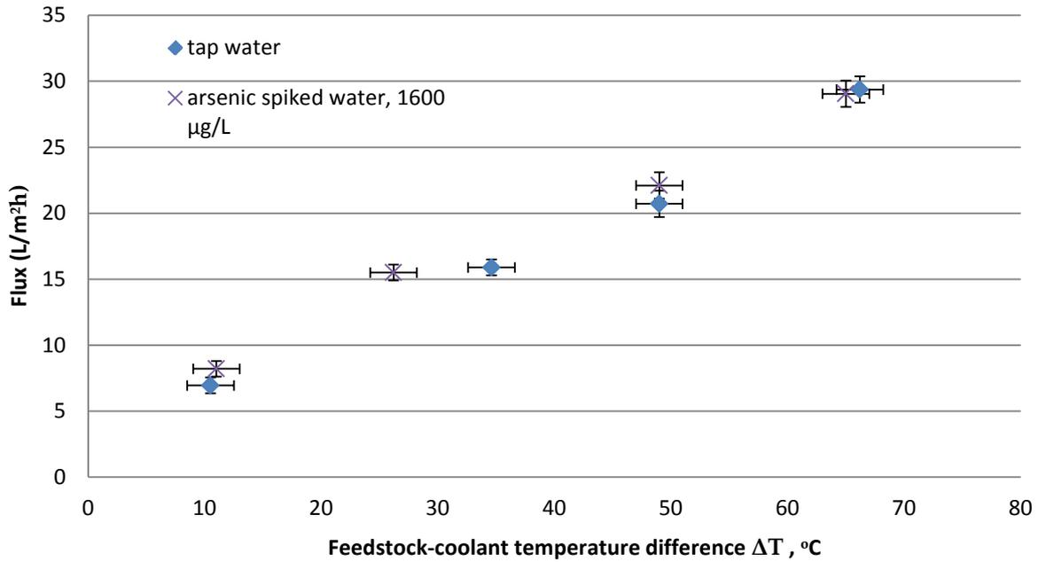
**Figure 3-2: Product water flux as a function of temperature difference across the membrane (feed water flow 3.8 L/min, coolant flow 1.9 L/min, feedwater inlet temperature ca 80 °C, coolant inlet temperature varying)**
