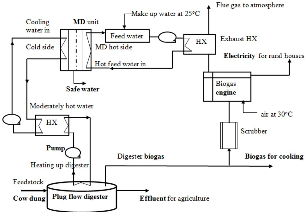
*Figure 4-1: Integrated systems for electricity, cooking gas and safe water production*
