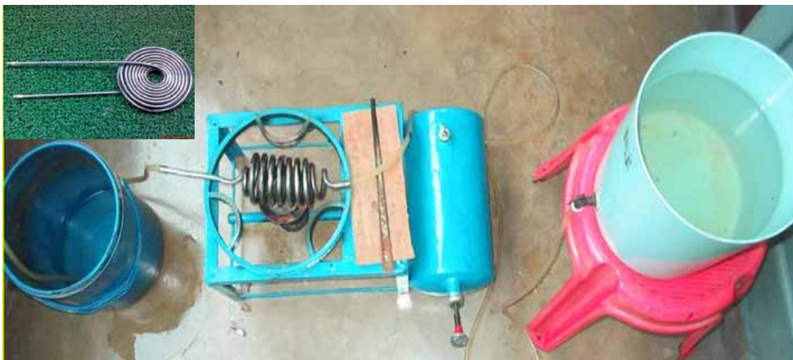
Figure 11: A shock killing system for removing bacteriological contamination from dug-well water
