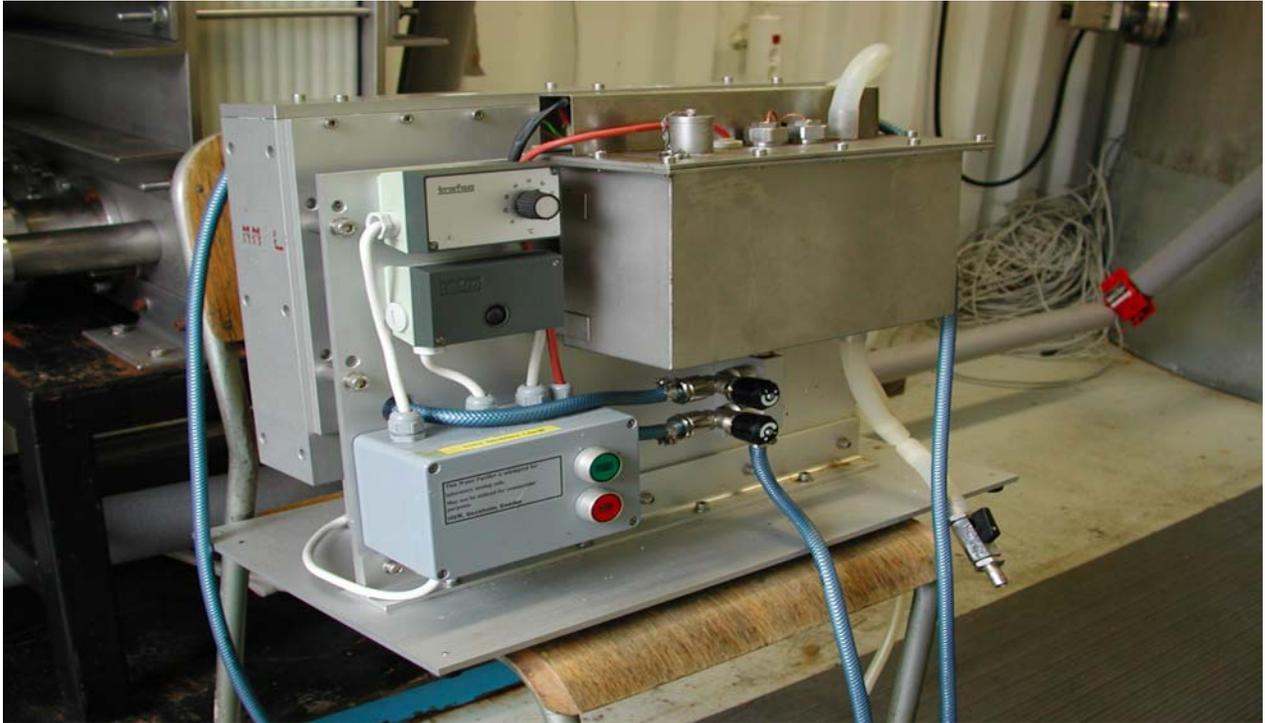
**Figure 16.** The lab unit of HVR water purifier (side view)
